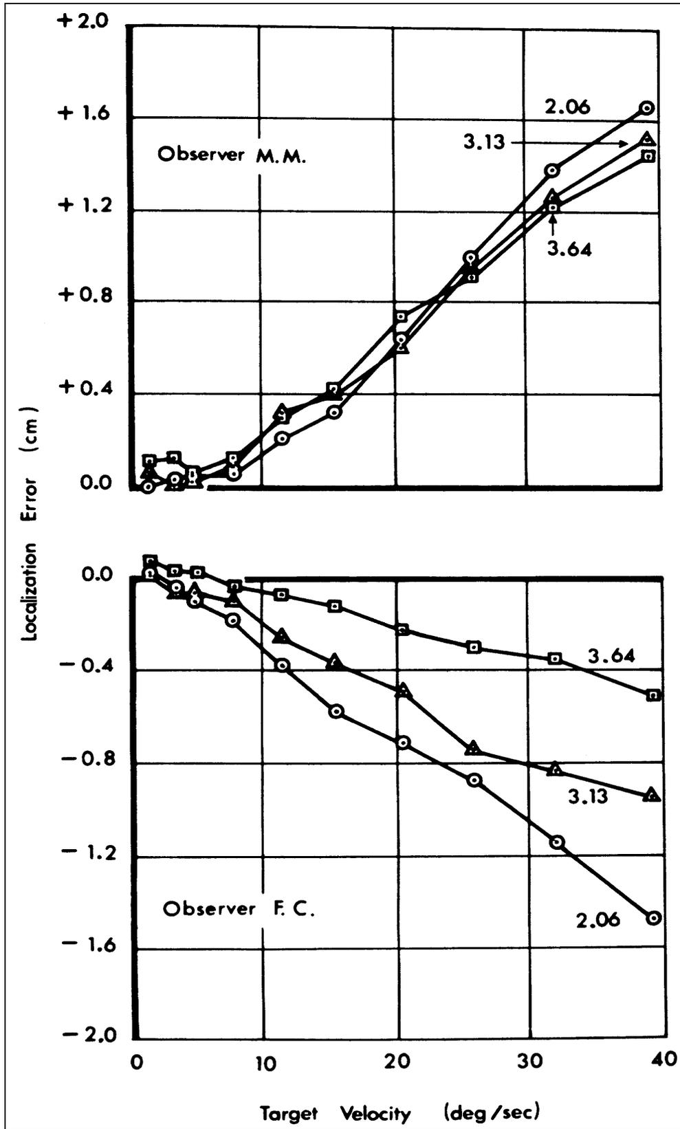
Fig. 2. Localization error of equidistance settings as a function of target velocity, with level of binocular retinal illuminance (in log trolands) serving as parameter.
