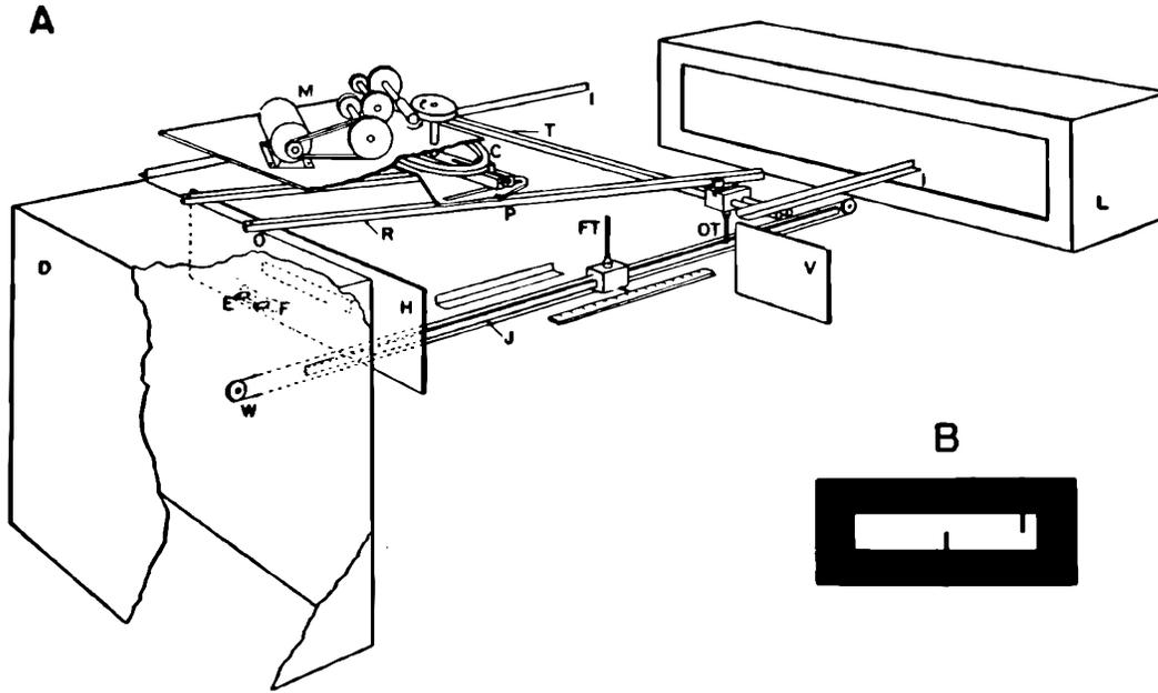
FIG. 2. Schematic representation of the apparatus and observer's view of stimulus targets. (a) The observer is seated in a dark room (D) and binocularly observes the fixation target (FT) located in the lower visual field and the oscillating target (OT) located in the upper visual field through a pair of artificial pupils (E). Movement of
