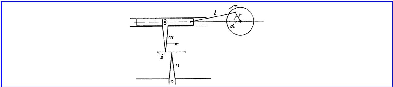
Fig. 3. Mechanism of Pulfrich's second model.
